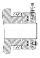
Screw the locking ring to the nut body, release pressure and work in completed
