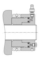
Screw the hydraulic nut to the upper end of the tightened bolt.
