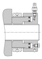
When the piston is jacked up, the bolts are stretched.
